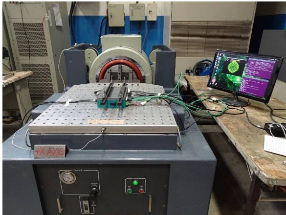
FIG 7.1: +X axis direction mounted
