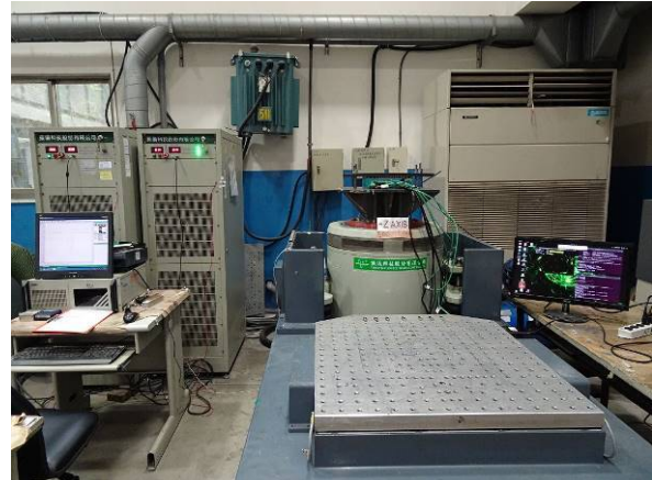
FIG 17.2: -Z axis direction mounted
