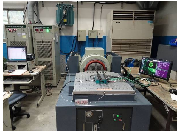
FIG 9.2: -X axis direction mounted
