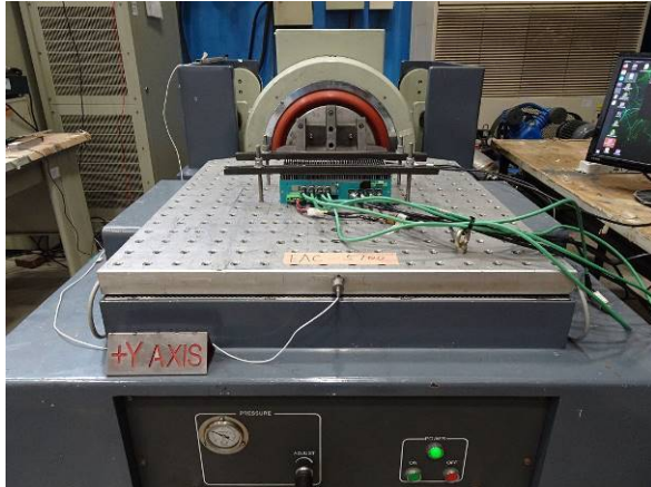
FIG 11.1: +Y axis direction mounted
